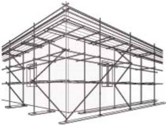
Typical independent tied scaffolding.
